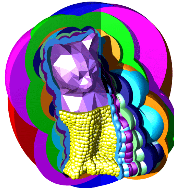
Wrapped BVH: a BV bounds its associated primitives, but not necessarily its child BVs
