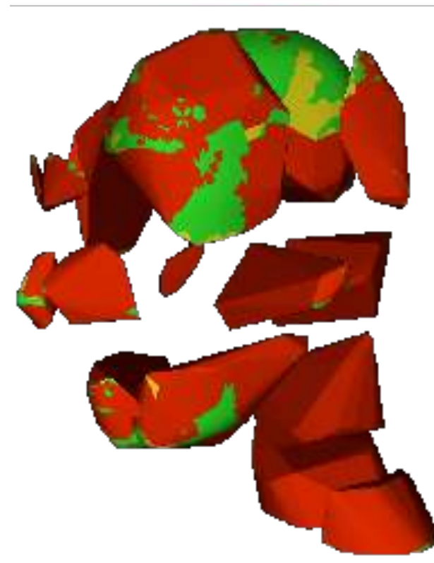
Convex pieces at a medium level of the hierarchy (green = orig. surface, red = free surface, yellow = "contained")
